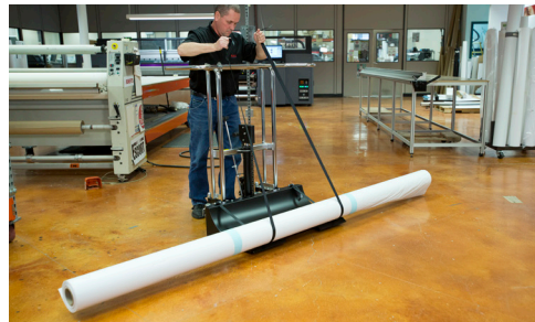
Got heavy rolls? Use the frame as a fulcrum to pull them onto the tray with minimal effort.
