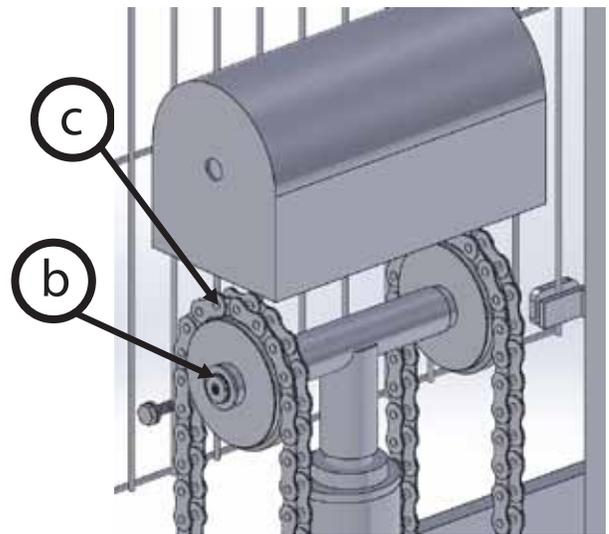
Remove screw to access the chain guide.
