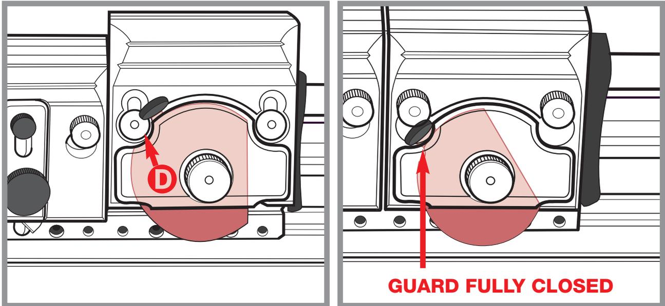
First raise the Cutter Bar using either Lift & Hold Lever, then loosen both of the Hinge location screws until the underside of the screw clears its location recess. Push the Cutter Bar until the underside of the location screw is positioned over the middle recess and tighten Hinge location screws. Repeat at the other end. The Cutter Bar is now positioned over the plastic Cutting Strip.
