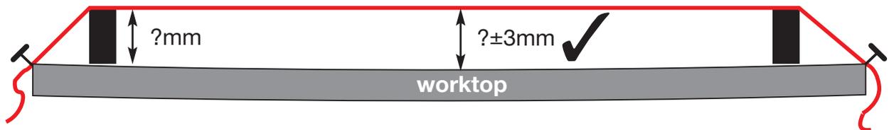
Adjust the surface flatness by adding packing pieces made from 1.5mm - 3mm (1/16" - 1/8") thick rigid material such as PVC Foamboard, under the Base Mounting Brackets as they are installed (next section).
