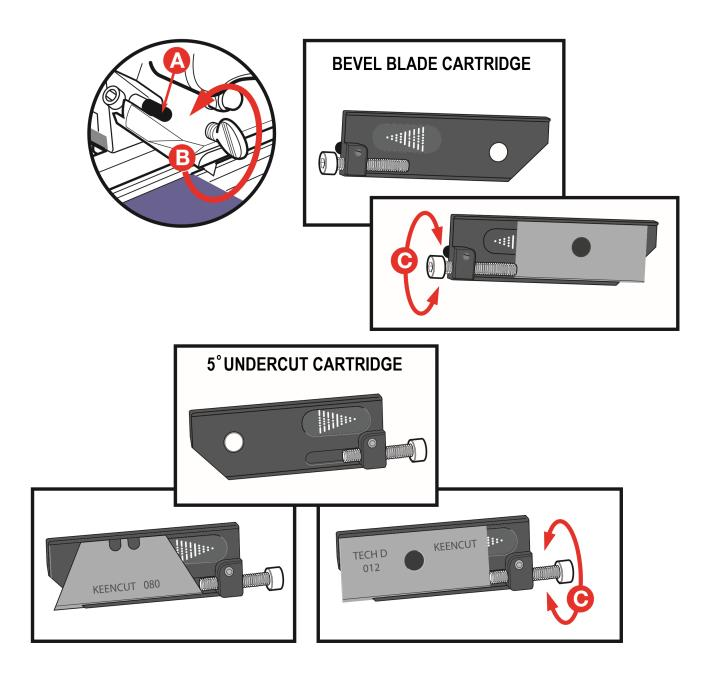
Both the bevel and 5° undercut blade holders are fitted with Blade Cartridges, to release the cartridge from either of the blade holders slacken the blade clamping screw (B) and pull the cartridge out, gripping the black plastic pin (A).
